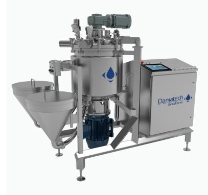
into the mixer below liquid level and instantly wetted. The powerful, high shear mixer and scraper agitator generates a controlled vortex in the tank. The combination of vortex and vacuum effectively separates air from the liquid and generates a perfect homogenous dispersion within seconds. The unit comes with an isolated jacket for fast heating and cooling with steam or ice water. For extra quick heating the unit is equipped with a direct steam valve.
