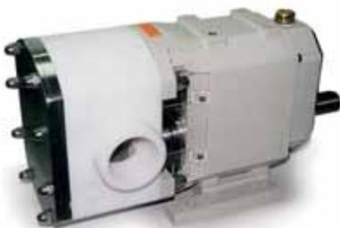
OMAC can produce Lobe pumps for transferring all kinds of aggressive products. The B100 and B330 Models can be manufactured in mixed versions, i.e. shafts and rotors in Titanium, Hastelloy or Monel, with the pump/cover body in Thermoplastic Resin. For larger sizes or high working pressures there are other
