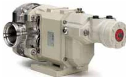
Specifically designed for road tanker duties, the B325, B330 and B390 can be supplied with flanged gear cover direct coupled to hydraulic motor. These pumps can be supplied bare shaft or complete with hydraulic motor, power station and control system.
