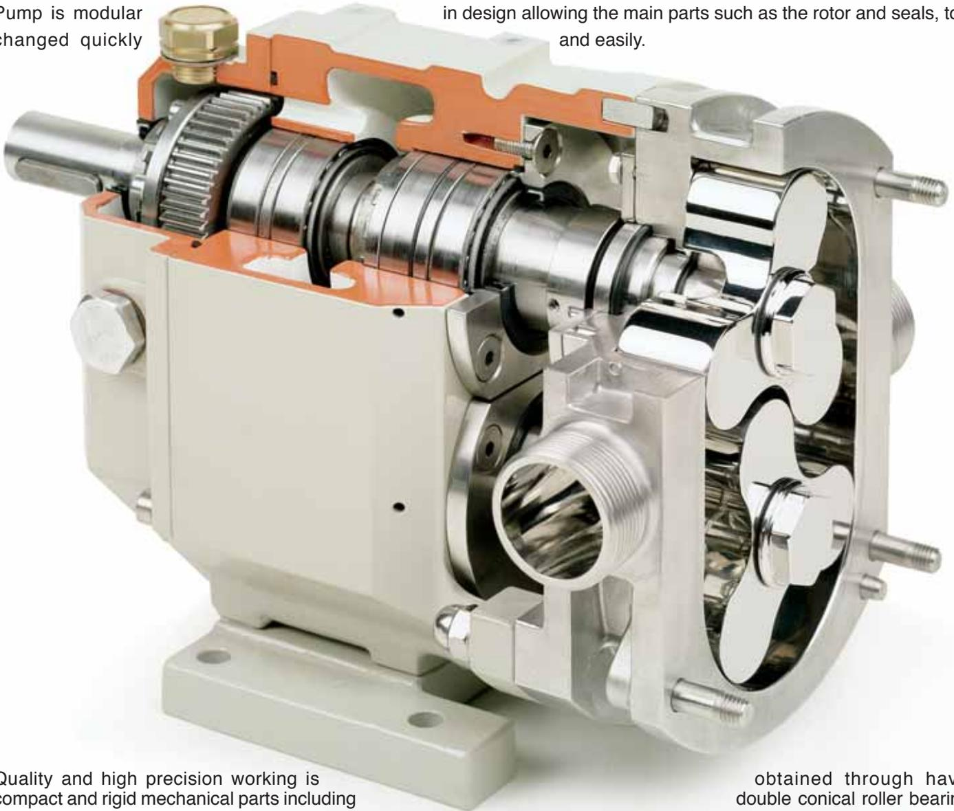
Quality and high precision working is compact and rigid mechanical parts including shafts and oversized gears running in an oil bath within This is to obtain smaller tolerances as the rotors do not have any contact points. This ensures a good pump performance and reliability is obtained.
