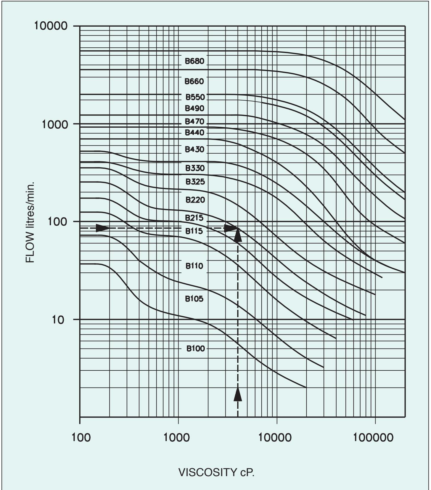
The curves on this chart define the fields of operation of the various sizes of pump, enabling a preliminary selection to be made according to viscosity/flow.
