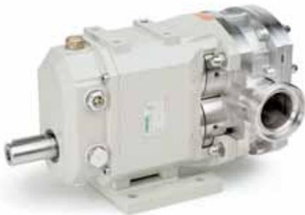
When the pump is transferring products that may crystallise or leave solid deposits, the mechanical seals supplied have to be cleaned by flushing water or a compatible liquid at low pressure. This flushing arrangement can also be used to dissipate heat or to avoid dry running. There is a fixed chamber around the standard seal with the UM seal for sealing the flushing liquid.
